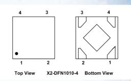
PIN1 - Vout, PIN2 - GND, PIN3 - EN, PIN4 - Vin
